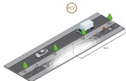
Optique P, 16 LED, 3700lm, 25W, 4m
